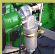
Oil change pump for routine oil change
