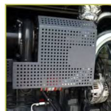
Heat and rotating part guards to prevent injuries to the user
